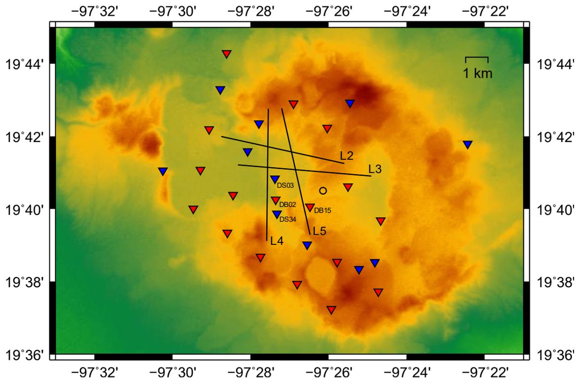
**Figure 1: Topographic map of the centre part of Los Humeros showing broad band (red triangles), and short period (blue triangles) seismic station locations, the four active-source vintage seismic lines L2-L5 and the location of well H-27 (black circle).**
