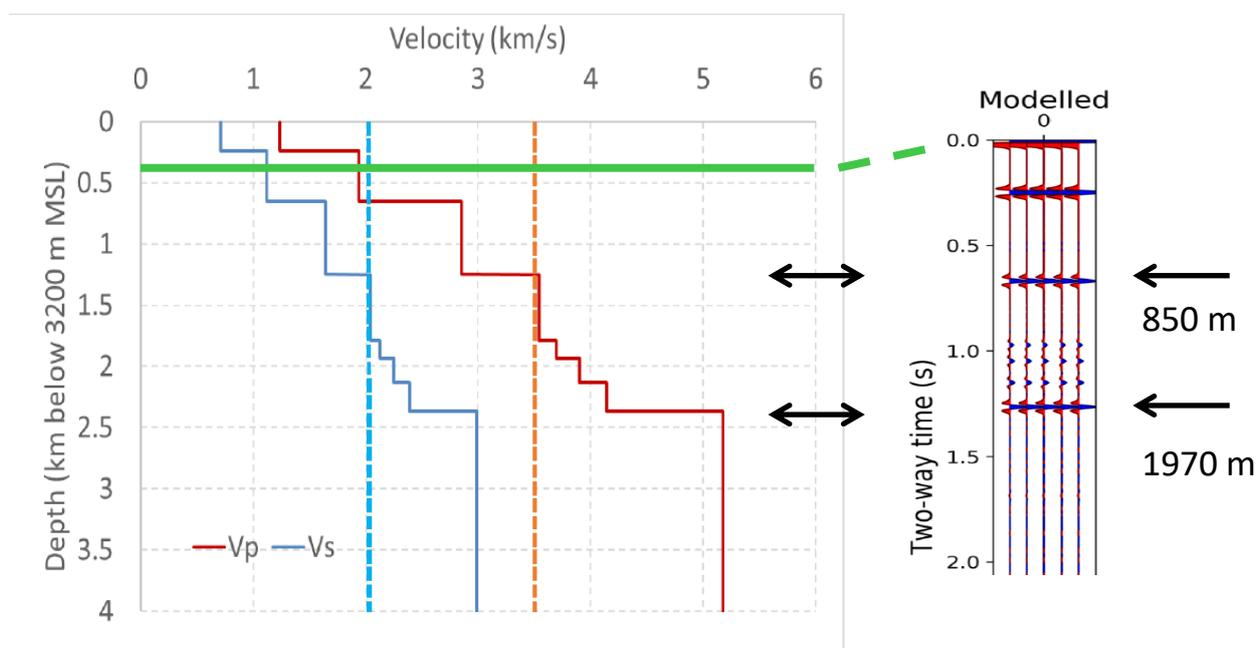
**Figure 2: Left: 1D P-wave (red) and S-wave (blue) blocky velocity profiles derived from seismic data at a location close to well H-27 (see Figure 1). A constant  $V_p/V_s$  is assumed: 1.732. After Hurtado (2001) and Lermo (2001). Right: FD-modelled reflectivity trace with 15 Hz Ricker wavelet and density taken constant at  $2.85 \text{ g/cm}^3$ .**
