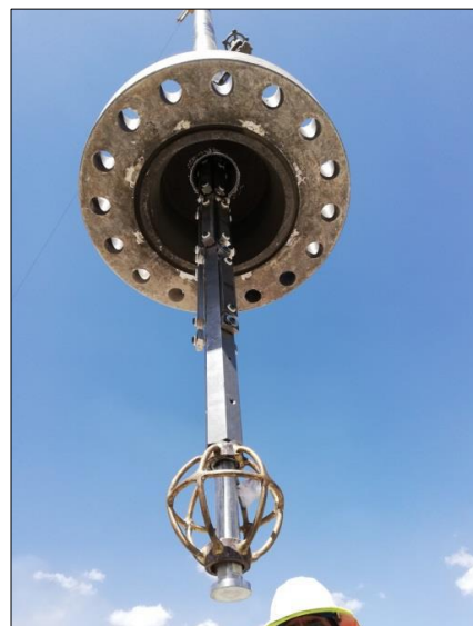
Figure 7. Preparations at well head for lowering the hexagonal sample holder with samples downhole. Pictures from CFE.
