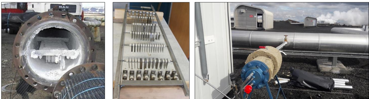
Figure 1. Surface testing. On the left steam pipe to the silencer with sample rack as shown in the middle picture. On the right corrosion tank with steam inlet from the main steam pipe.
