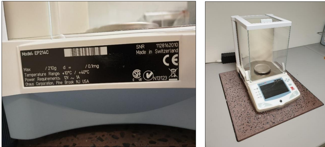
Figure 15. Precision scale, OHAUS Explorer Pro EP214C, used for weight loss measurement.
