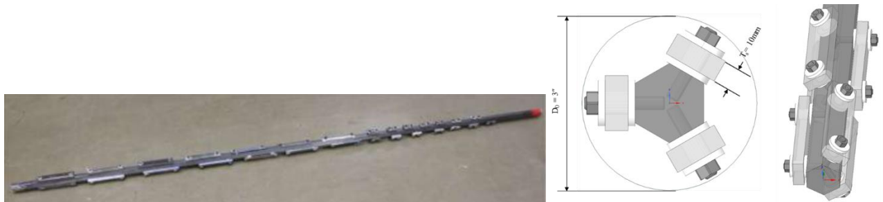
Figure 2. Sample rack for downhole testing. Hexagonal bar with attached samples on the left ready for downhole testing in well in Iceland (Karlsdottir and Thorbjornsson 2013). On the right drawing showing how ceramic washers are used to ensure no metal to metal contact between sample and test bar.
