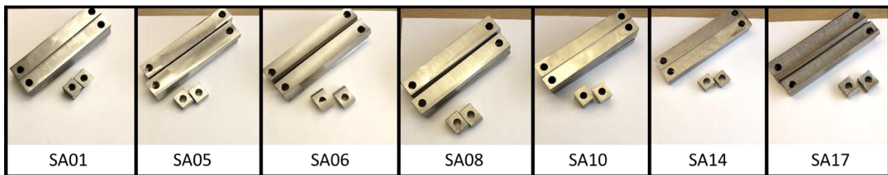
Figure 5. Figure showing the samples used in Los Humeros. Three larger specimens and two smaller of each material was used for downhole testing.
