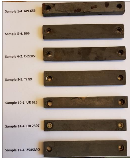
Figure 9. Samples as received from testing. Samples for XRD analyses were taken from scaling on sample 1-4, 5-4, 14-4 and 17-4.
