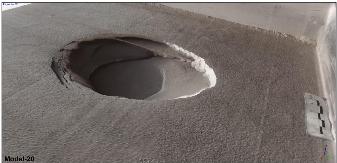
Figure 3.18. 3D reconstruction (using Agisoft Photoscan®) of Model-20 showing the rectilinear feature derived from the reactivation as normal fault of an inherited fault. The latter was introduced before model deformation as a brittle discontinuity in an internal and near-tangent position with respect to the analogue magmatic chamber.
