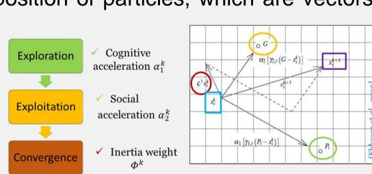
PSO algorithm: position and velocity update at k+1 iteration
