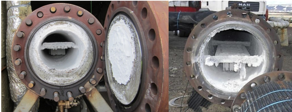
Figure 4: Heavy silica scaling in the surface equipment of the IDDP-1 well during discharge testing (Karlsdottir et al., 2015).
