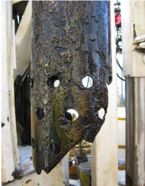
Figure 3: Heavy corrosion of liner pipe in the KJ-39 well (source: deliverable D4.3 from GeoWell project, Thorbjornsson 2016).
