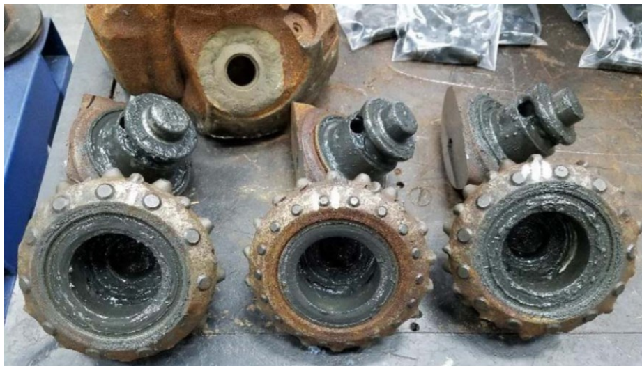
Figure 6: Cones and bearing from high-temperature tri-cone roller cone drill bits used during drilling of the IDDP-2 well in the Reykjanes geothermal field in Iceland (Stefánsson et al., 2018).
