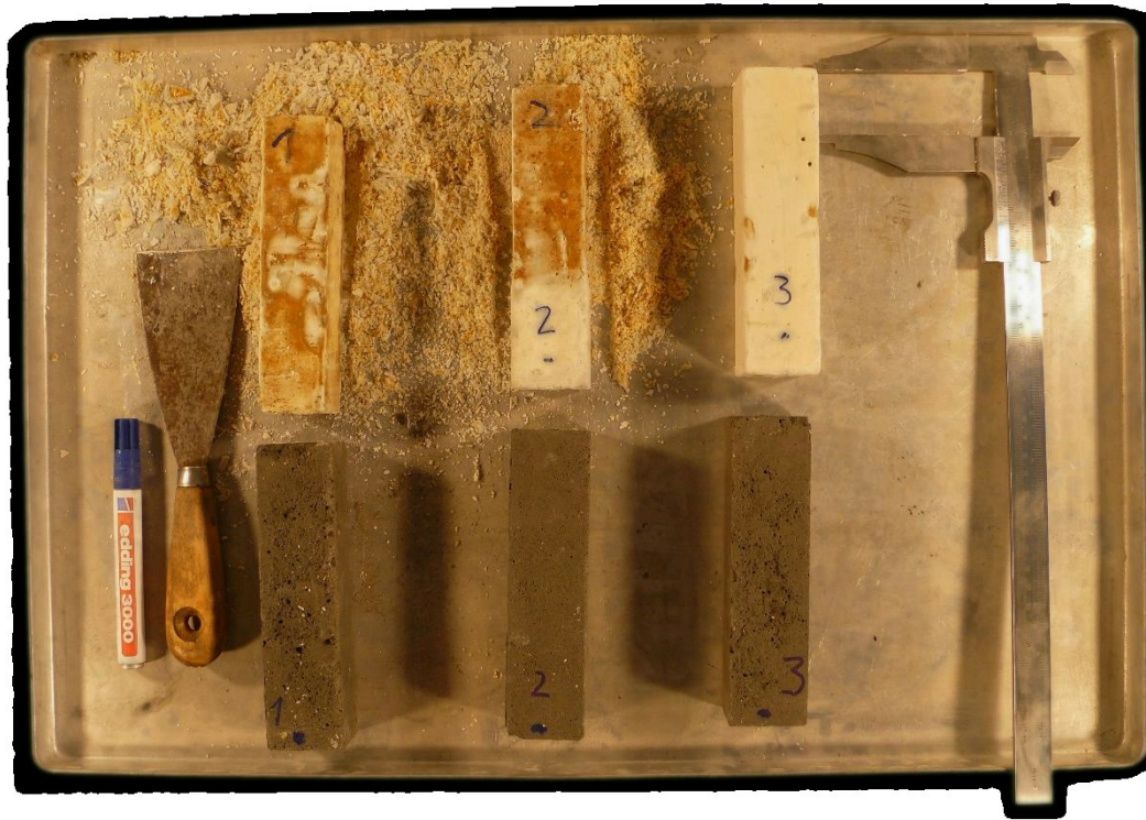
Figure 20: Results of 7 days of an “acid bath” in a 6% HCl solution (upper row – OPC samples, lower row – geopolymer samples).
