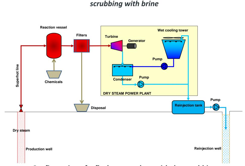
*Configuration of a flash steam plant with dry scrubbing*
