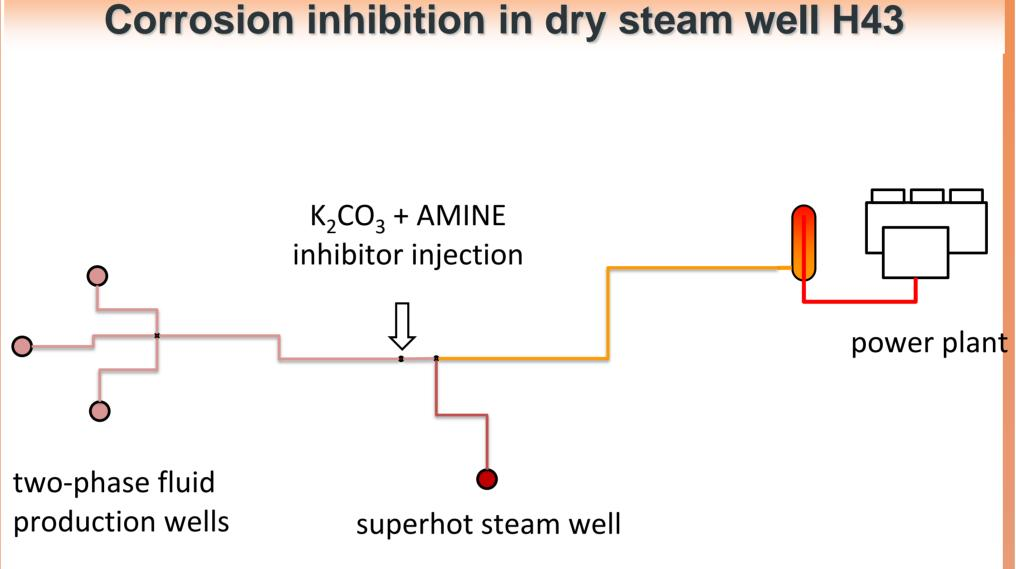
In Los Humeros, injection of inhibitors at the two phase line before the intersection of the H43 steam line, effectively mitigated corrosion allowing the integration of superheated steam wells into the power
