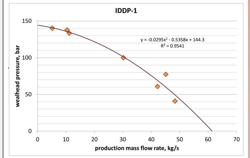
A 5-7 km deep well drilled in Los Humeros is expected to have similar production features with well IDDP-1 as an approximation
