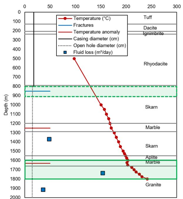
Figure 21: Temperature and lithology in EAC-1. The most promising stimulation targets are the Marbles and Granites below 1600 m (solid green) based on a temperature anomaly and fluid loss. Open hole stimulation will likely stimulate the well directly below the casing (dashed green).
